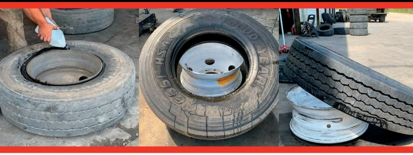
Murphy's Off The Rim Bead Breaker is the perfect lubricant for easing tires off the rim by penetrating between the beads and tire flanges. Our fast acting formula will break through even the toughest beads.
